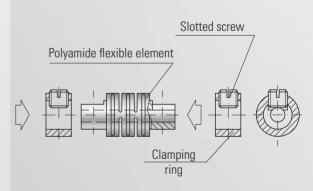
The set screw is securely guided through the clamping ring, which is partially supported by the flexible element. The set screw contacts the shaft directly.
