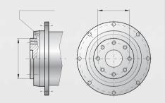
The bolt circle will be machined to match the gearbox
