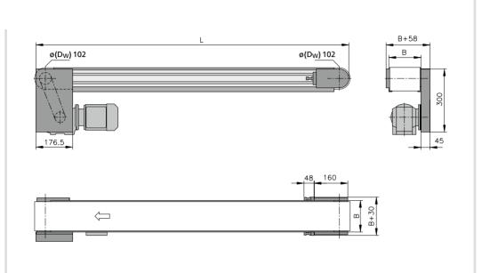
Use of timing belts with fixtures possible with this drive version. When using cams, the max. possible height must be requested.
