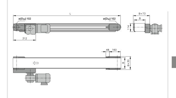
The overall height of the drive assembly is held to an absolute minimum. The timing belt pulley ensures outstanding transmission of the motor power. Use of timing belts with fixtures is possible without restriction with this drive version.
