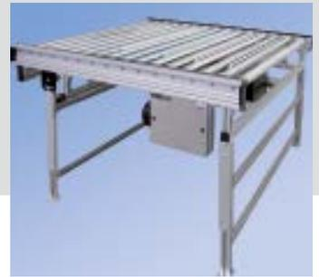
The roller conveyor, RBT-P 2255 with a tangential chain drive is used wherever long conveyor sections with motor drive are required. Drive occurs via a ½" chain, which in an encapsulated durable wear strip, drives the conveyor rollers on a tangent from below via a sprocket. The tangential roller conveyor can
