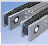
Chain Conveyor System KTF-P 2010 is designed for the transport of heavy pallets. The different chain and Wear strip options make for an extremely low-maintenance and robust conveyor. The wear strips have a low coefficient of friction, and provide good wear
