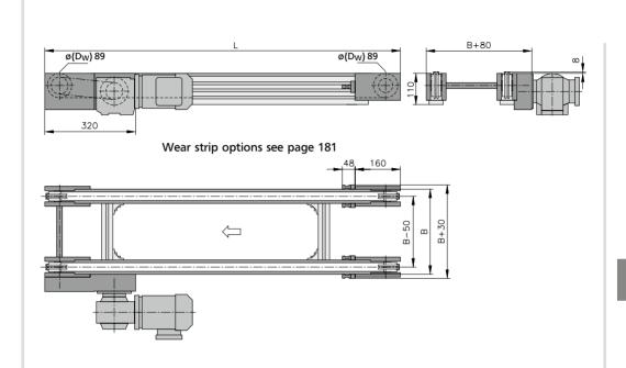
The overall height of the drive assembly is held to an absolute minimum. Use of attachment chain is not possible with this drive version.
