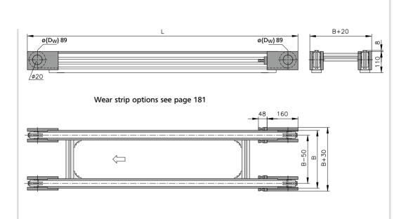
The AA drive variant, offers the advantage of operating multiple conveyor strands in parallel or in series with one drive. Depending on the requirement, the conveyor is designed either with a hollow shaft or with a connecting shaft with shaft journal (ø 20 mm, usable length 34 mm, incl. feather key DIN 6885) Operation with cleats is not possible with this version.
