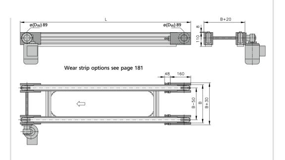
By placing the motor directly onto the drive shaft, this drive version minimizes not only the space required at the drive yet also the number of moving parts and maintenance requirements. Use of attachment chain is not possible with this drive version.
