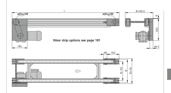
The sprocket ensures outstanding transmission of the motor power. Use of attachment chain is not possible with this drive version.
