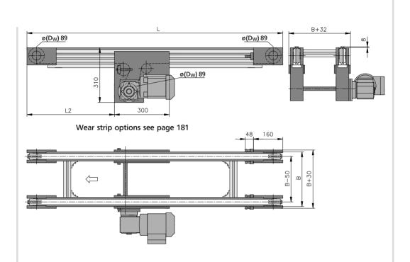
Thanks to the motor fitted directly onto the drive shaft, for this drive version, the spatial requirements and the maintenance effort are reduced to a minimum. The compact conveyor frame structure, and the possibility of freely selecting the drive position over the entire length of the conveyor, facilitate integration of the conveyor in existing systems. The travel direction is reversible. Operation with cleats is not possible with this version.
