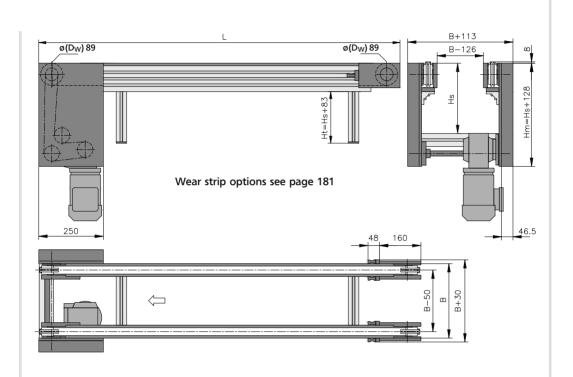
In principle, the drive concept of the AQ version is the same as for the AC version. This drive is used when the goods to be transported or the pallets require a free space between the conveyor strands. Operation with cleats is not possible with this version.
